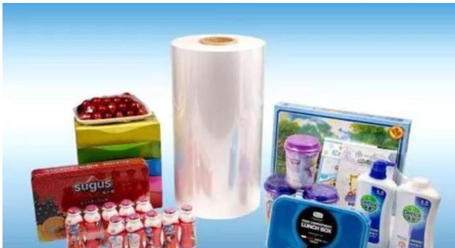
POF full name multi-layer co-extruded polyolefin heat-shrinkable film, which uses linear low density polyethylene as the intermediate layer (LLDPE), copolypropylene (PP) as the inner and outer layers, plasticized and extruded through three extruders, then processed by special processes such as die forming and bubble inflation. It is a new type of environmentally-friendly shrink film, which is the most widely used and rapidly developed in the world.
